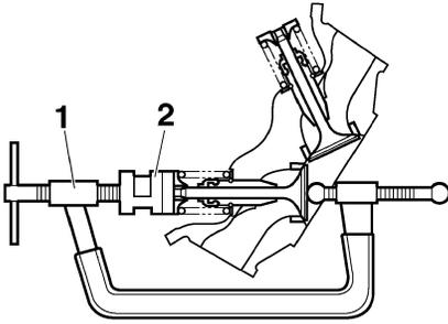
5. To secure the valve cotters onto the valve stem, lightly tap the valve tip with a soft-face hammer.
