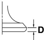
Valve stem diameter (intake) 4.475–4.490 mm (0.1762–0.1768 in)
