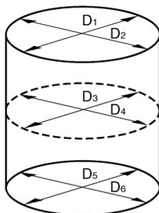
b. If out of specification, rebore or replace the cylinder, and replace the piston and piston rings as a set.
