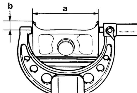
b. 10 mm (0.39 in) from the bottom edge of the piston
