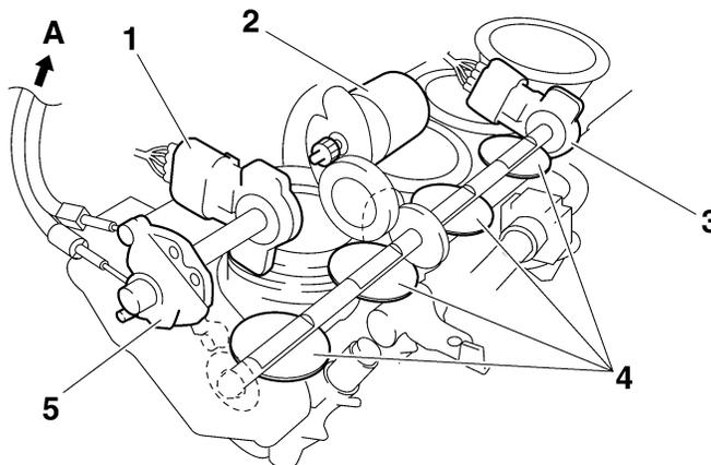
1. Throttle position sensor (for throttle cable pulley)
