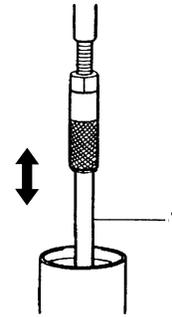
13. Before measuring the fork oil level, wait ten minutes until the oil has settled and the air bubbles have dispersed.
