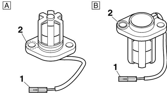
b. Measure the oil level switch resistance.
