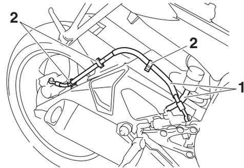
3. Hold the vehicle upright and apply the brake several times.
