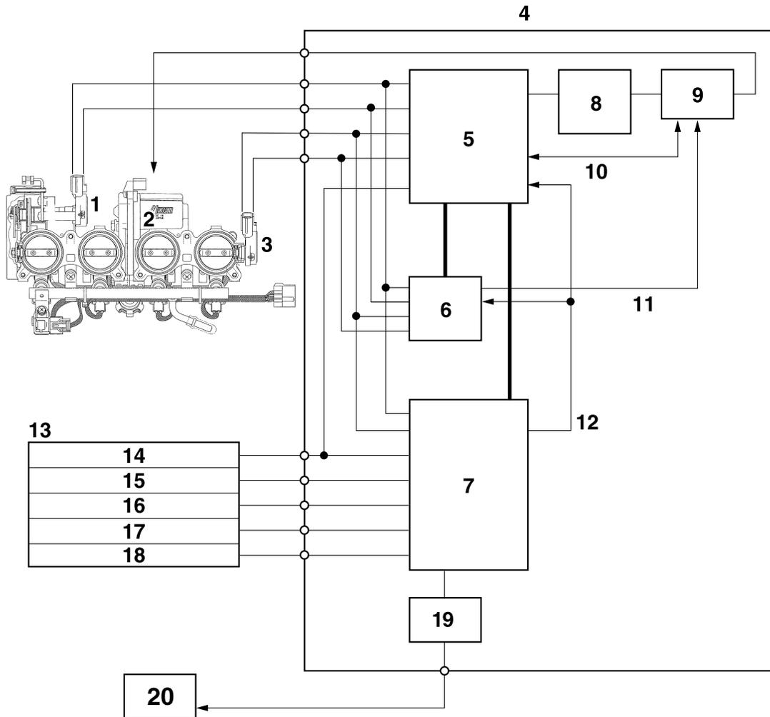
1. Throttle position sensor (for throttle cable pulley)
