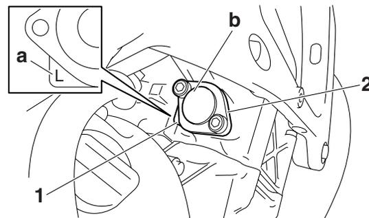
6. Rotate the crankshaft a few times to release the timing chain tensioner rod.
