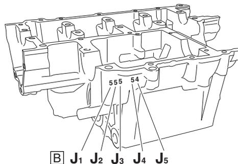
For example, if the crankcase J<sub>1</sub> and crankshaft web J<sub>1</sub> numbers are 6 and 2 respectively, then the bearing size for J<sub>1</sub> is:
