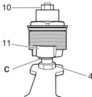
o. Remove the rod holder and fork spring compressor.
